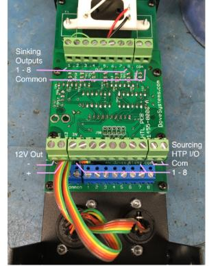
application with the Dove PR43, the DE8's DIP switches for Option 1 and Option 2 (see <u>On/</u><u>Off Output Options</u> section below) will be set ON so the DMX can control the 4 relays independently.
